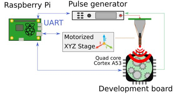
Fig. 2. EM pulse injection setup
