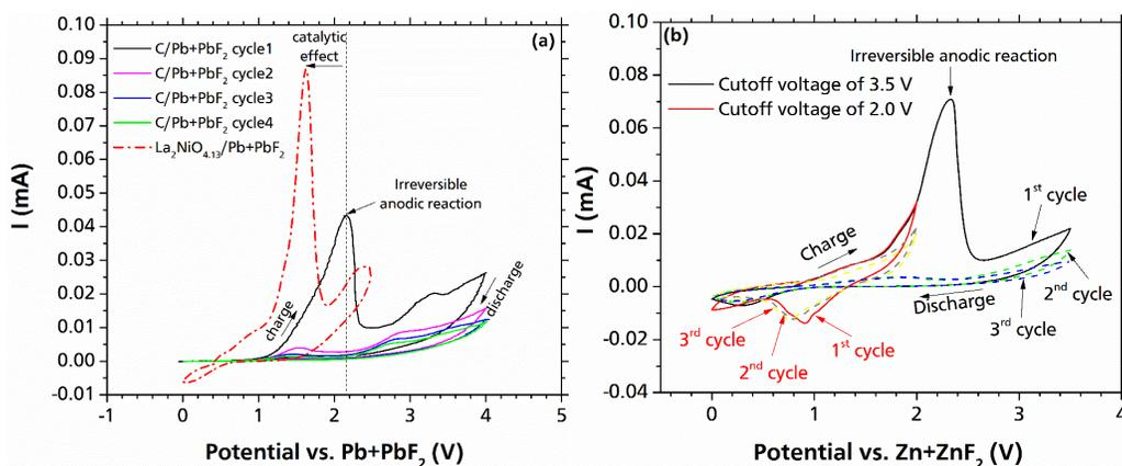
Figure 24. Cyclic voltammograms of a carbon electrode as compared to  $La_2NiO_{4+d}$  cathode material ( $Pb+PbF_2$  as counter electrode); (b) Cyclic voltammograms of  $La_2NiO_{4+d}$  cathode material vs.  $Zn+ZnF_2$  in two different potential range of 0 – 2 V and 0 – 3.5 V. Figures are reproduced with some modifications from ref.<sup>27</sup>.
