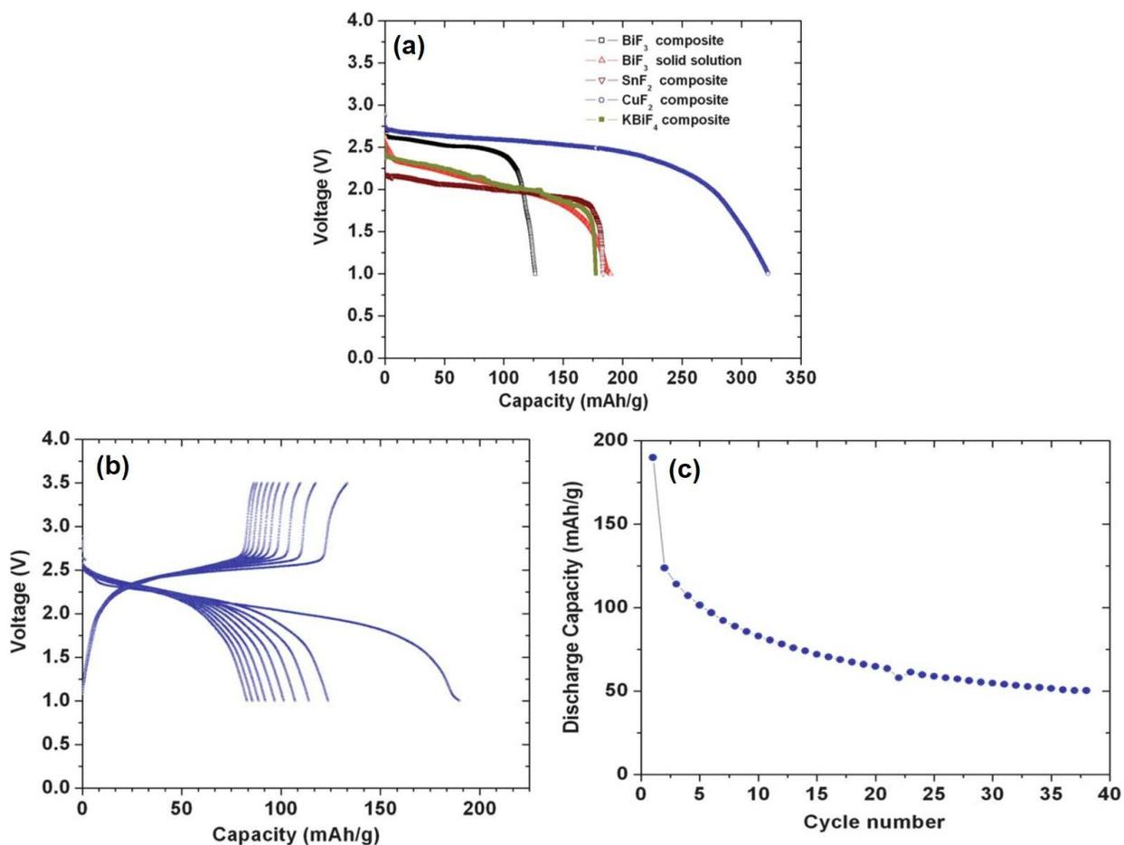
Figure 14. (a) Voltage-capacity profiles of various metal fluorides vs. Ce metal. The discharge curves were obtained at 150 °C with a current density of 10 mA/cm<sup>2</sup>; (b) Cycling performance of the BiF<sub>3</sub> (solid solution)/Ce cell for the first 10 cycles; (c) changes of discharge capacity with cycle numbers for the same electrochemical cell. The figures have been reproduced from ref.<sup>8</sup> with permission <sup>xiv</sup>.
