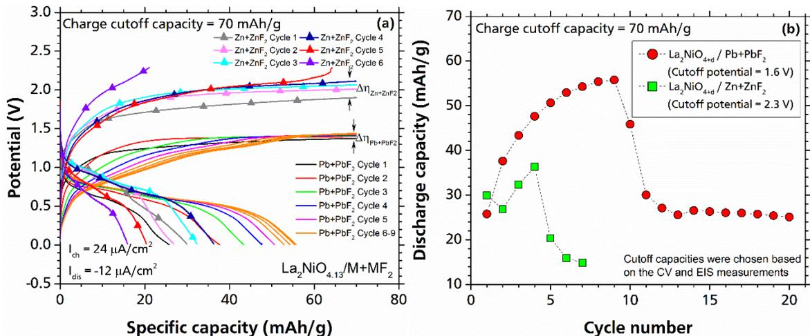
Figure 18. The effect of anode material on the overpotential and cycling behavior of  $\text{La}_2\text{NiO}_{4+d}$  by showing (a) the first few cycles of  $\text{La}_2\text{NiO}_{4+d}$  against  $\text{Zn}+\text{ZnF}_2$  and  $\text{Pb}+\text{PbF}_2$  anode materials (b) discharge capacities of  $\text{La}_2\text{NiO}_{4+d}$  against  $\text{Zn}+\text{ZnF}_2$  and  $\text{Pb}+\text{PbF}_2$  anode materials. Reproduced from ref.<sup>151</sup>.
