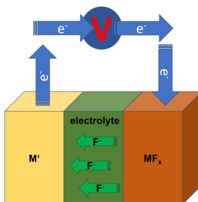
Figure 2. A schematic illustration of the metal/metal fluoride conversion based FIB proposed by Reddy and Fichtner<sup>8</sup>.
