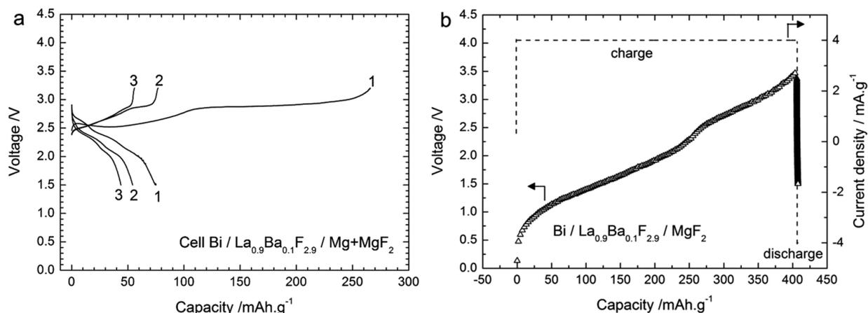
Figure 15: Voltage profiles of the first three cycles of a cell  $\text{Bi/La}_{0.9}\text{Ba}_{0.1}\text{F}_{2.9}/\text{Mg}+\text{MgF}_2$  (a) and of the first charging and discharging of a cell  $\text{Bi/La}_{0.9}\text{Ba}_{0.1}\text{F}_{2.9}/\text{MgF}_2$ . The cells were heated to  $150\text{ }^\circ\text{C}$ , a current density of  $4\text{ mA.g}^{-1}$  ( $10\text{ mAcm}^{-2}$ ) was applied. (The figures have been reproduced from ref.<sup>23</sup> (an original RSC publication)).
