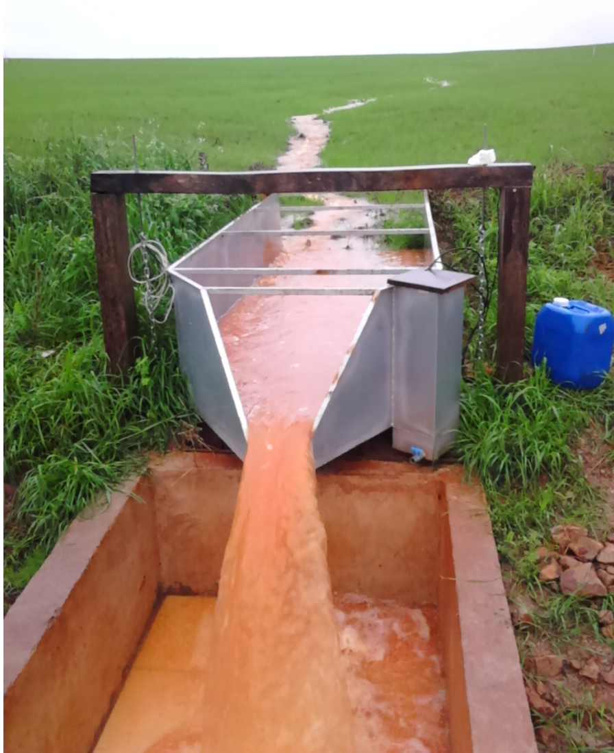
Figure 3. H-flume for monitoring the flow rates installed in the lower part of the catchments and macroplots.
