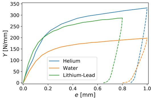
Figure 3: Individual characteristic curves of the three HELICOFLEX® seals giving the linear load as a function of the seal compression. Solid line: compression curve; dashed line: unloading curve.
