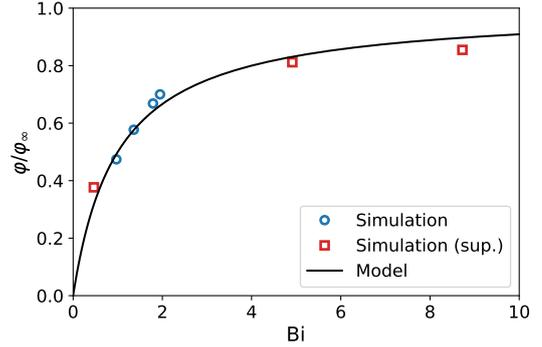
Figure 6: Dimensionless water cooling heat flux as a function of the Biot number of Eq. (6). Blue dots: simulations varying  $h_c^1$ ; red squares: supplementary simulations varying both  $h_c^0$  and  $h_c^1$ ; solid line: model of Eq. (5) with  $\varphi_\infty = 5$  kW (best fit).
