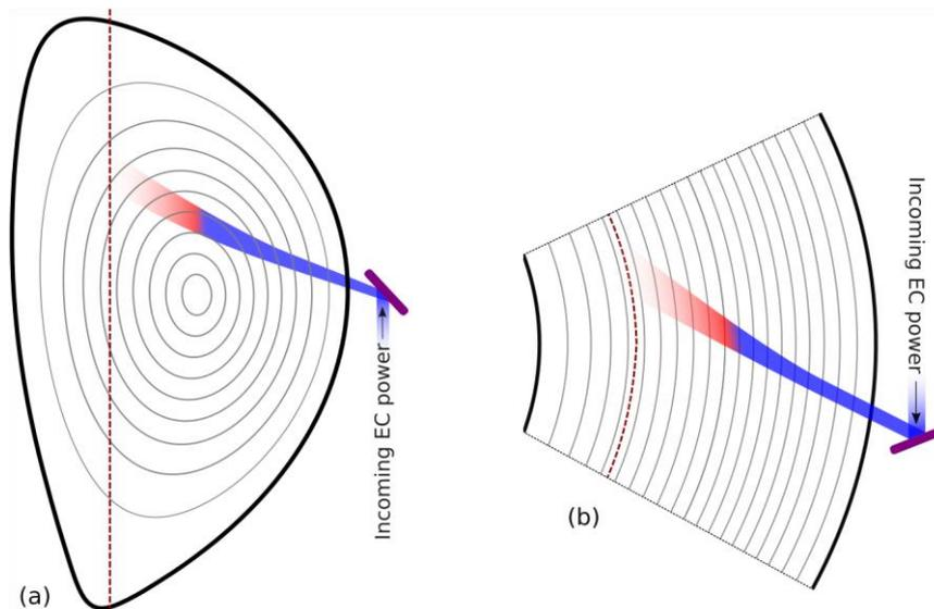
Figure 5: Schematic of EC wave heating and current drive in a tokamak such as ITER. (a) Poloidal cut; (b) Top view. The beam is shown in blue, with red colouring at locations where significant absorption occurs. The (fictitious) EC steering mirror is shown in magenta, and is used in this representation to inject the wave with a toroidal angle with respect to the magnetic field direction, a situation typical of ECCD. The red dashed curve shows the cold EC resonance.
