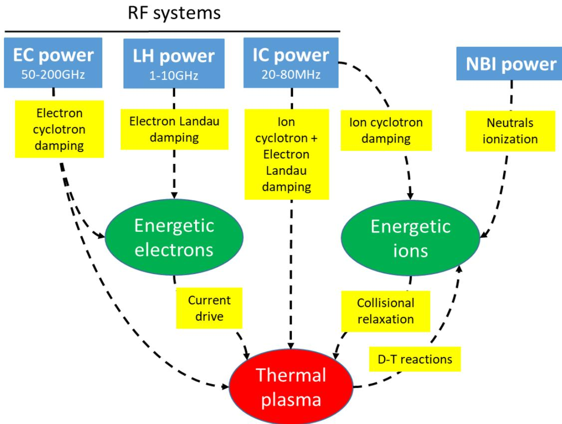
Figure 1: Summary of the main heating and current drive sources in modern magnetically confined fusion plasmas.
