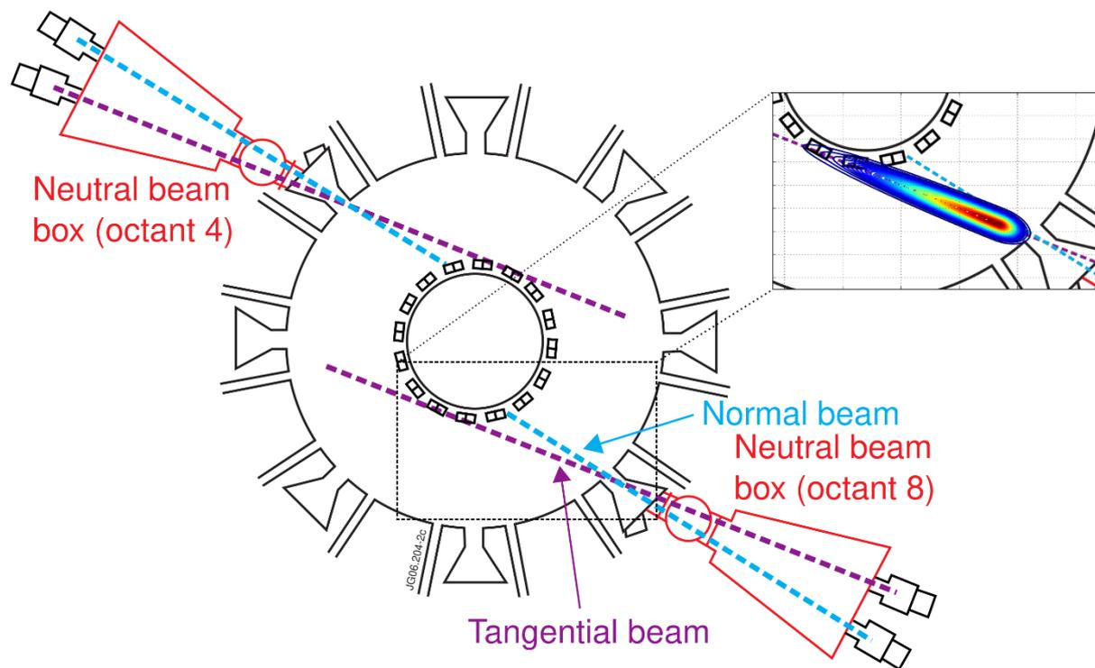
Figure 2: NBI heating in the JET tokamak. This device is equipped with two separate NBI injectors located in octants 4 and 8, each consisting of eight beams arranged in a tangential bank and a normal bank (Source: EUROfusion). In the inset is shown an illustration of the power deposition profile in the plasma corresponding to the tangential bank of the injector located in octant 8.
