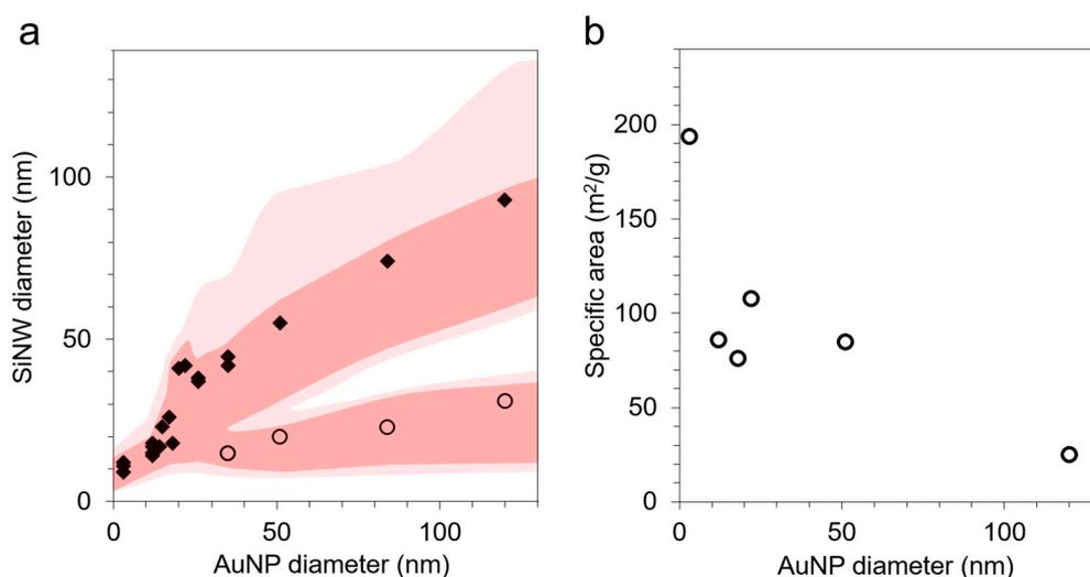
**Figure 4.** (a) Average diameter of the main (diamond) and minority (circles) SiNW populations as a function of the size of the catalyst AuNPs, as measured by SEM (diameter histograms in Figure 3 and Figure S3). The shaded zones show the full width at half maximum and the 90% limit for both SiNW diameter peaks. (b) Specific area of the SiNWs as measured by the BET method as a function of the size of the AuNP catalysts.
