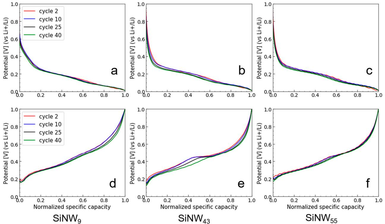
**Figure 8.** Normalized galvanostatic curves in lithiation (a–c) and delithiation (d–f) as a function of the cycle numbers for SiNW<sub>9</sub> (a,d), SiNW<sub>42</sub> (b,e), and SiNW<sub>55</sub> (c,f).
