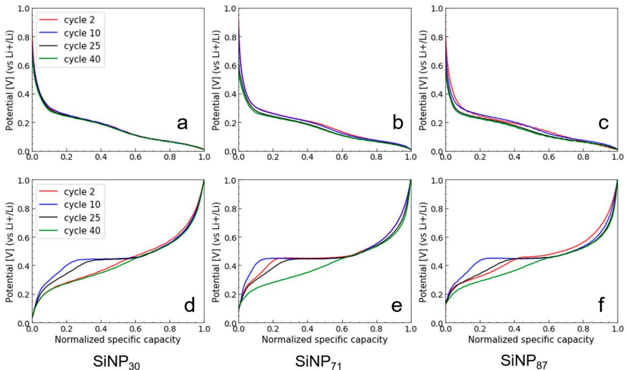
**Figure 7.** Normalized galvanostatic curves in lithiation (a–c) and delithiation (d–f) as a function of the cycle numbers for SiNP<sub>30</sub> (a,d), SiNP<sub>71</sub> (b,e), and SiNP<sub>87</sub> (c,f).
