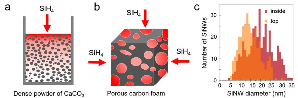
**Figure 2.** Scheme of the partial pressure reduction in the porous growth support,  $\text{CaCO}_3$  powder (a) and carbon foam cube (b). The  $\text{SiH}_4$  pressure is represented in red shades. (c) Diameters of Si nanowires (SiNWs) grown from 1–2 nm gold nanoparticles (AuNPs) in a  $1\text{ cm}^3$  carbon foam cube on the surface (“top”) and 2 mm below the surface (“inside”). Inside, SiNWs had the same diameter distribution at all depths down to the center.
