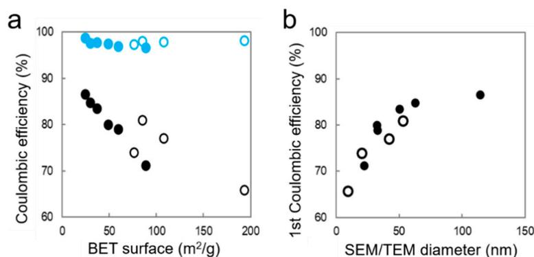
**Figure 6.** Coulombic efficiency as a function of BET specific area (a) and statistical SEM/TEM diameter (b) for SiNPs (full circles) and SiNWs (empty circles) on the 1st cycle (black) and the 5th cycle (blue).
