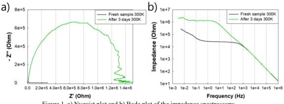
Figure 1. a) Nyquist plot and b) Bode plot of the impedance spectroscopy.
