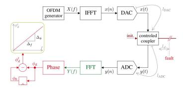
Fig. 7. Schematic diagram of the novel cable diagnosis system using a single FFT block to analyze the phase of the reflected reflectometry signal and locate a fault using the variation of the phase versus the variation of the frequency.
