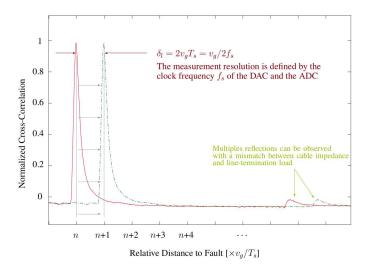
Fig. 3. Two reflectograms illustrating the spatial resolution  $\delta_l$ . The measurement error of a fault location over a CUT is always lower than  $v_g/T_s$  meters, which is represented by the length difference between solid red and dashed-green reflectograms.
