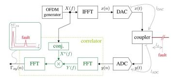
Fig. 1. Schematic diagram of a standard OMTDR based cable diagnosis system using a correlator between the injected signal x(n) and the reflected signal y(n) to detect the location of a fault in a CUT.
