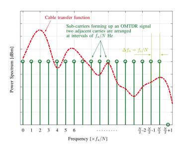
Fig. 2. Positive part of the spectrum of an OMTDR signal  $X(f_n)$  with N sub-carriers (green) and the cable frequency-domain transfer function (red) defined in the same band as the multi-carrier signal, i.e.,  $f_s/2$  with  $f_s$  being the DAC sampling frequency.
