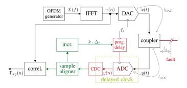
Fig. 4. Schematic diagram of an OMTDR based cable diagnosis system using a correlator between the injected signal x(n) and the received signal y(n) to detect the location of the fault. The acquisition resolution is improved through a pseudo oversampling achieved using a constant phase-shift increasing on the sampling clock of the ADC.
