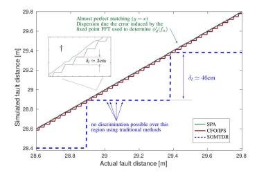
Fig. 8. Computational simulation comparison between the estimated and actual fault location for a standard coaxial EN WZFRF15 CUT after applying the SOMTDR correlation-based reflectometry and the IPS, CFO and SPA techniques. † Zoom around 29m.
