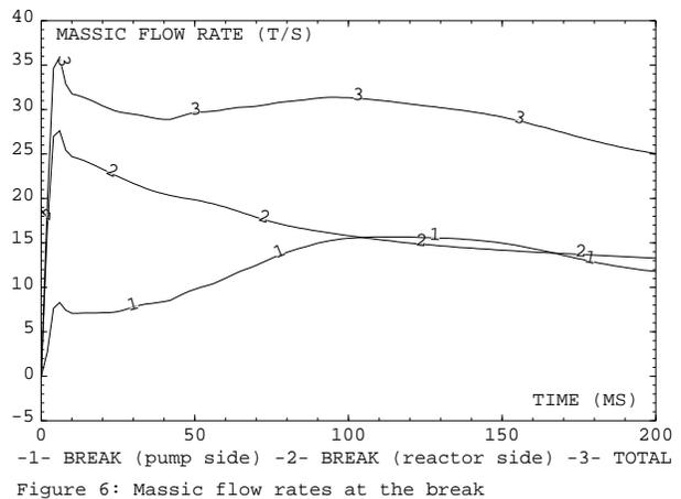
Figure 6: Massic flow rates at the break
