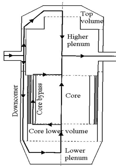
Figure 2: The pipe model for the reactor
