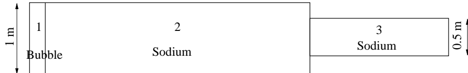
Fig.4: Equivalent shock tube with a section change
