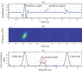
Fig. 12. Experimental results of TFDR. (a) TFDR measured signal. (b) Time–frequency distribution of the measured signal. (c) Time-frequency cross-correlation value. From [145].
