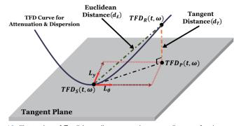
Fig. 13. Illustration of Euclidean distance and tangent distance for time-frequency distributions. From [142].
