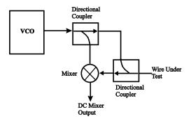
Fig. 10. PD-FDR Block Diagram. From [132].
