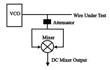
Fig. 11. MSR Circuit Diagram. From [136].
