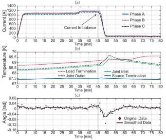
Fig. 14. Results of the current imbalance induction test. (a) Current profile. (b) Temperature profile. (c) Time-frequency phase spectrum at the joint box. From [100].
