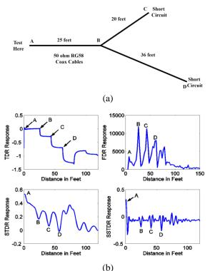
Fig. 1. (a) A network of RG-58 cables and (b) their measured responses using TDR, FDR, STDR, and SSTDR. From [85].
