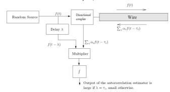
Fig. 6. NDR Type I Block Diagram. From [121].
