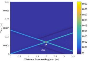
Fig. 15. A space-time ZT diagram of a single Y-junction network showing the voltage propagation after applying DORT method where a focal spot can be on the position of the soft fault. From [159].
