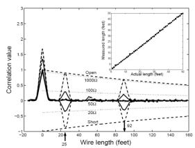
Fig. 8. Measured correlation of NDR Type II for 25 and 92 foot RG-58 (50  $\Omega$ ) wires with resistive terminations. The inset shows the measured vs. actual length measured using an open circuited 18-gauge paired wire. This shows excellent linearity between the peak location and wire lengths. From [121].
