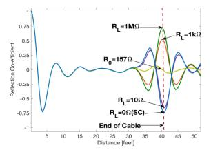
Fig. 2. SSTDR response of different resistors connected at the end of the 40-foot PV cable. The dashed red line in the figure denotes the end of the cable. From [95].
