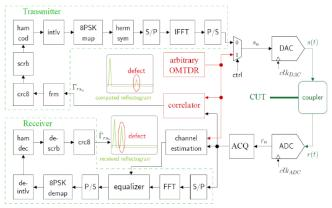
Fig. 5. A schematic diagram of sensor communication based on OMTDR technology. From [113].
