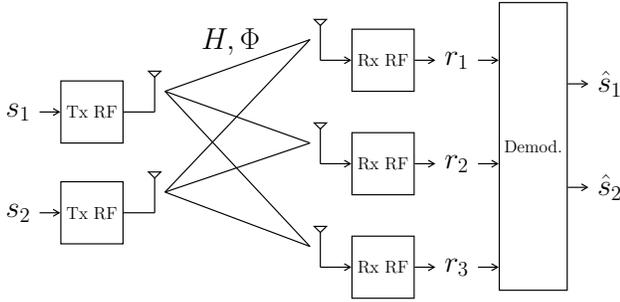
Fig. 1: Block diagram of a  $2 \times 3$  MIMO transceiver
