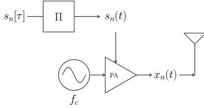
Fig. 2: Block diagram of one Tx RF chain
