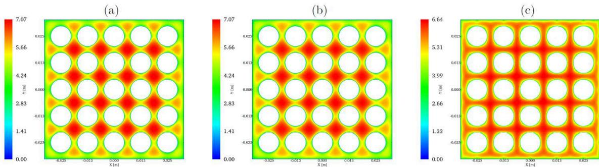
Fig. 6: Inlet axial velocity in m/s. (a) LEVM, (b) NLEVM, (c) LES.
