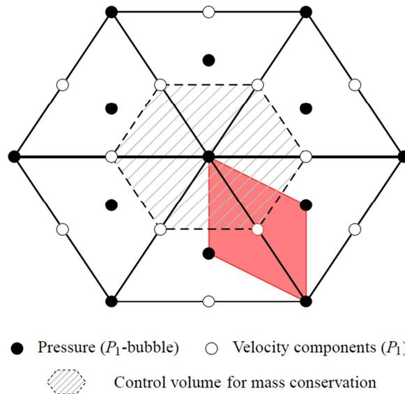
Fig. 3: Schematic 2D representation of the FVE discretization method in TrioCFD with respective positioning of degrees of freedom and control volumes.
