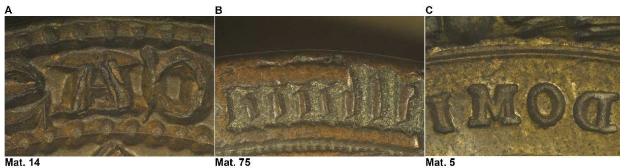
194 Figure 4 : Different techniques to realise the letters on the seal matrices: (A) engraving, (B) simple stamps combination, (C) 195 letter-punches 196
