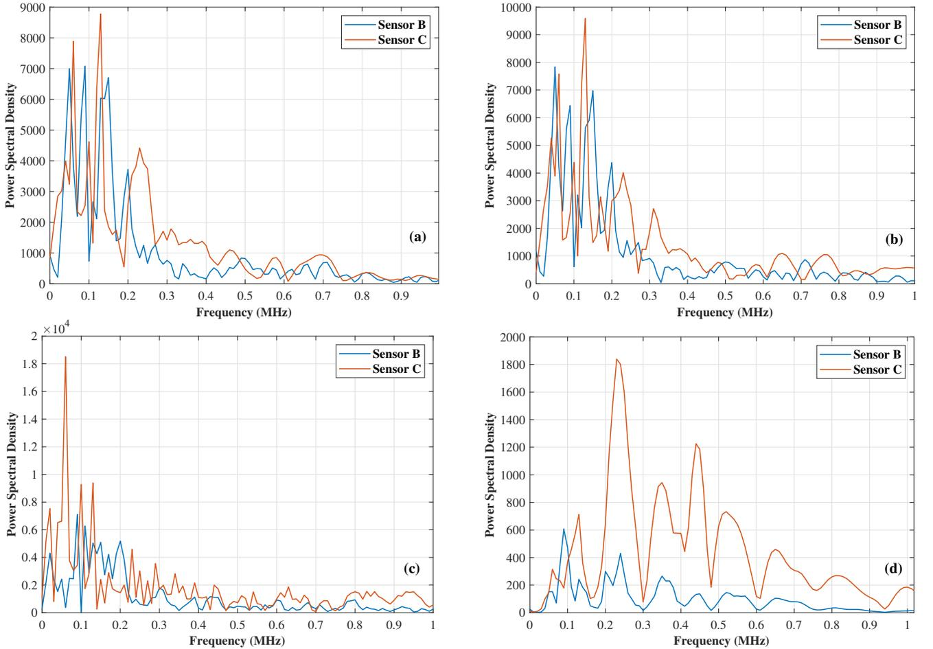
Fig. 6: Spectra of the FOTs as measured by sensors B and C for the faults triggered by: (a) CB and 30  $\Omega$  resistance, (b) CB and 60  $\Omega$  resistance, (c) CB with the spark ignitor, and (d) CB with the spark ignitor and a 60  $\Omega$  resistance.
