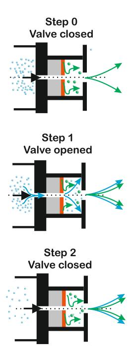
Figure 6. Scheme showing the flow of 2-HP molecules (in green) and carrier gas atoms (in blue) entering and leaving the oven at each cycle of the pulse valve.
