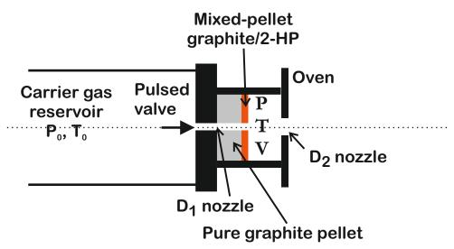
Figure 2. Not to scale scheme of the beam source (Pulsed valve + Oven).
