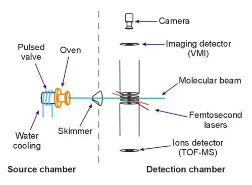
Figure 1. Experimental setup. In the present paper, the Time-of-Flight Mass Spectrometer (TOF-MS) is not used.
