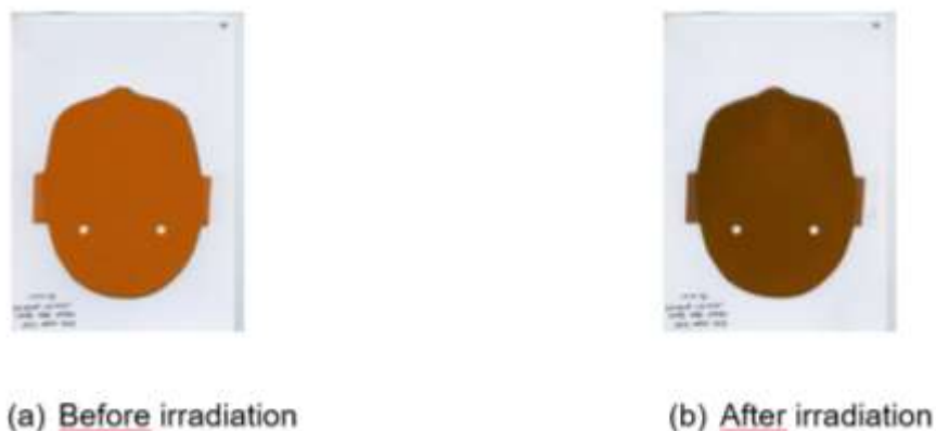
Figure 6: Film read-out for the head acquisition: the color of XR-QA films turns from orange to brownish-black.
