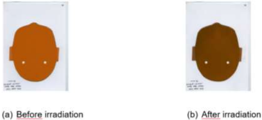
330 Figure 6: Film read-out for the head acquisition: the color of XR-QA films turns from orange to 331 brownish-black.
