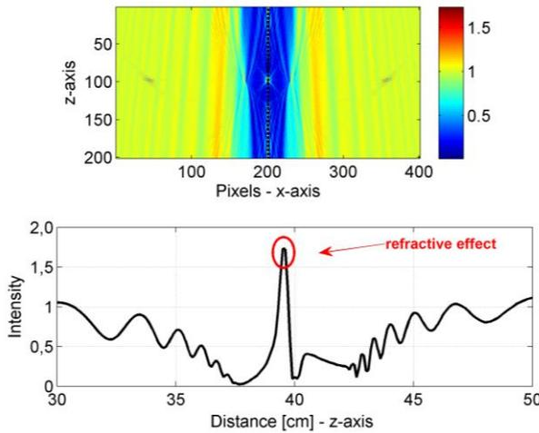
**Figure 1** Cross sections of modulus of the field reconstructed from simulations calculated with the generalized Lorenz-Mie theory (the section plane passes through the center of the droplet and contains the  $z$  axis) – Case of a 1 mm droplet observed at 40 cm,  $Nf \approx 3$ .
