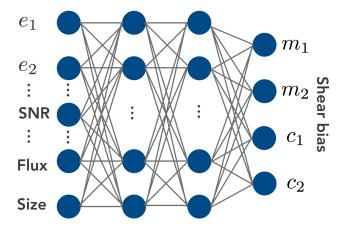
**Fig. 2.** Visual schema of the ML approach of the method. A set of measured image properties is used as input features for the neural network. The system is then trained to produce the shear bias parameters as output.
