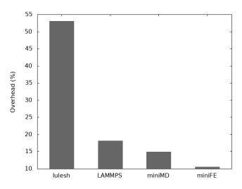
Fig. 2: Compilation-time overhead (ratio between the new PARCOACH analysis time and the total compilation time).
