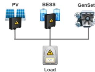
Fig. 5. application #2 - Hybrid microgrid topology
