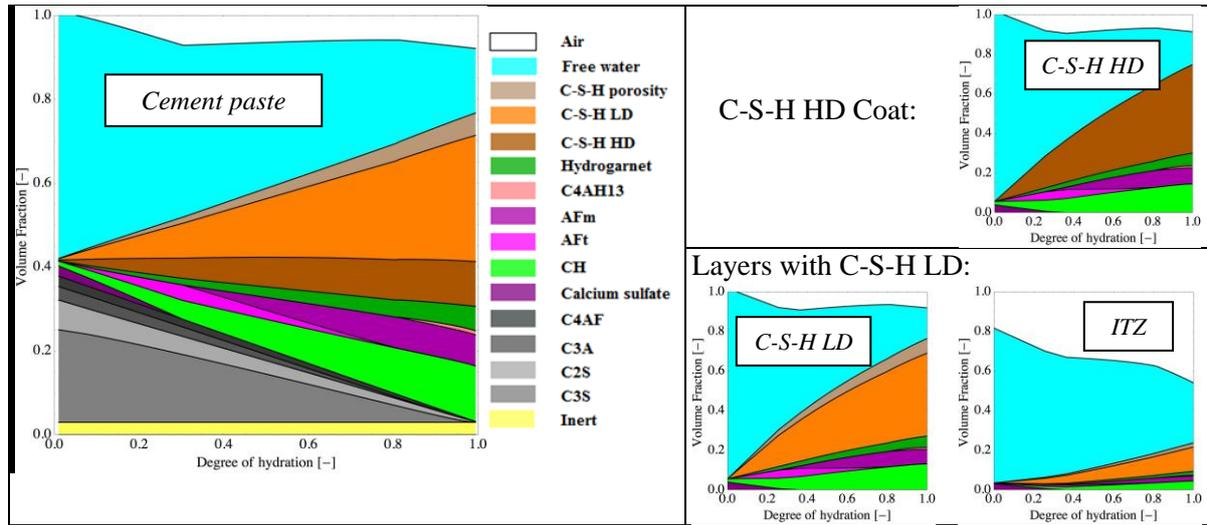
Figure 2. Volume fraction of the cement paste and different layers: C-S-H HD, C-S-H LD and ITZ
