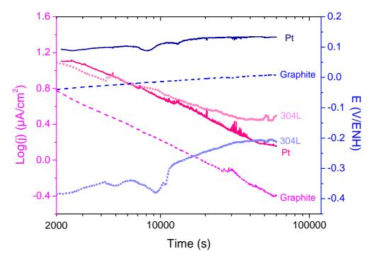
**Figure 7:** Potential and galvanic density current values as a function of time for Mg alloy coupled with Pt, graphite or 304L in ZRA mode after transient regime.
