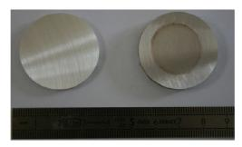
**Figure 8**: Mg alloy sample before (on the left) and after (on the right) galvanic coupling with graphite during 16h in 0.1M NaOH.
