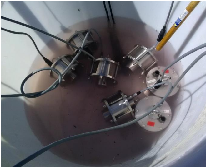
Calibration with several controled Rhodamine concentration
