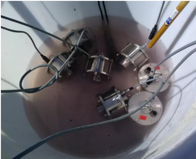
Calibration with several controled Rhodamine concentration
