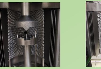
Tungsten furnace can heat up to **1800°C**
