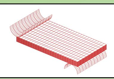
**Frederick-Armstrong law**<sup>[2]</sup> licos@Cast3m<sup>[3]</sup> code used for the numerical viscoplastic constitutive law with kinematic hardening describing primary creep
