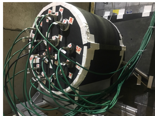
Figure 3: LOENIE long counter with its 16 ^3\text{He} detectors
