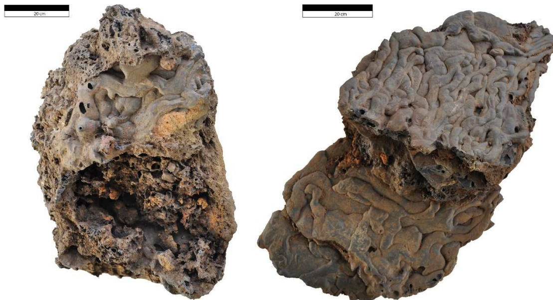
Figure 2: Examples of tap slag found on Angkorian archaeological sites from the Phnom Dek area.
