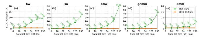
Figure 5: Simulation results of EDP reduction compared to the 512-bit SIMD. Each label is the CIM vector width used (in bit).
