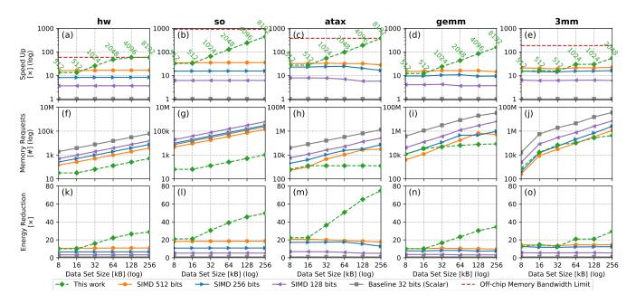
Figure 4: Simulation results of execution speed up, memory requests and energy reduction of five kernels, compared to the scalar architecture (RISC-V with SRAM). Each label (in *Speed Up*) represents the CIM vector width (in bit) for each data set size.
