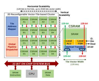
Figure 1: Reconfigurable Tiles of C-SRAM Architecture, integrated with a CPU on a standard system bus.
