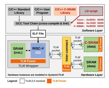
Figure 3: Hardware/Software Simulation Platform.
