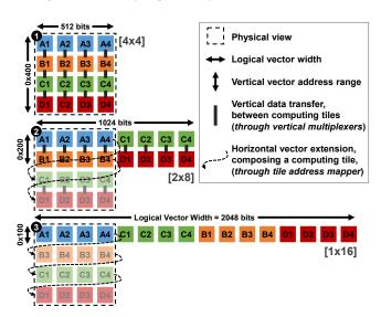
Figure 2: Physical and logical view for 3 vector configurations: **0** 512-bit, **2** 1024-bit and **3** 2048-bit wide.
