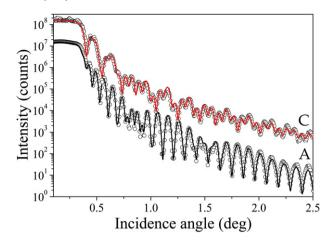
Fig. 7. XRR measurements (open circles) and fits (solid lines) of the as-deposited samples A and C at 8.05 keV.
