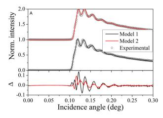
**Fig. 10.** Ag-K $\alpha$  GIXRF Gilda measurements and fits of sample A. The difference curve is represented at the bottom of the figure. Model 2 has been obtained by combining sets of data acquired at different excitation energies. It offers smaller differences between experimental and simulated data.
