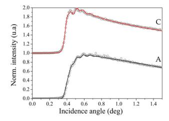
Fig. 8. Ag-L $\alpha$  GIXRF measurements (open circles) and fits (solid lines) of the as-deposited samples A and C at 8.05 keV.
