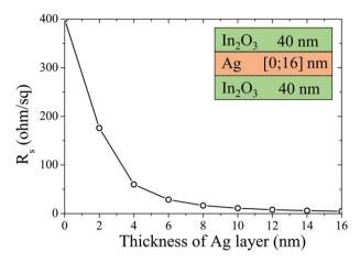
**Fig. 1.** Sheet resistance for IO/Ag/IO tri-layer samples with an Ag layer with varying thickness. 0 nm of Ag represents the sheet resistance of an 80 nm pure  $In_2O_3$  layer. For photovoltaic applications, acceptable sheet resistances have been obtained with Ag thickness superior to 4 nm.
