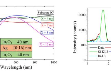
Fig. 2. Optical transmittance for IO/Ag/IO tri-layer samples with an Ag layer with varying thickness. For photovoltaic applications, the transparency in the visible is necessary and sample with an Ag thickness of 12 nm are not adapted.
