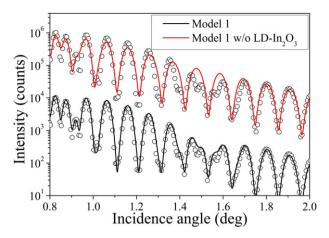
**Fig. 9.** XRR measurements (open circles) and fits (solid lines) of the as-deposited samples A at 8.05 keV with and without the introduction of the low-density  $In_2O_3$  top layer in the model. It can easily be seen that in order to reproduce the experimental data around 1.5°, the introduction of a low-density top layer is necessary.
