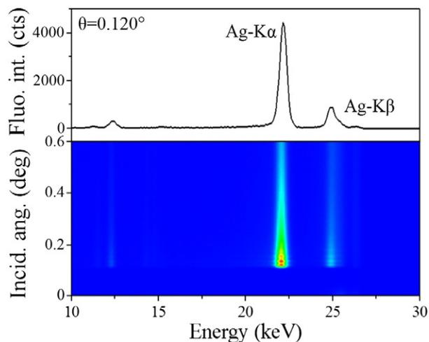
**Fig. 5.** Fluorescence intensity from a measurement at 26,400 eV with a synchrotron radiation at an angle of incidence  $\theta = 0.12^\circ$ . With this excitation energy, the fluorescence peaks of interest are not overlapping.
