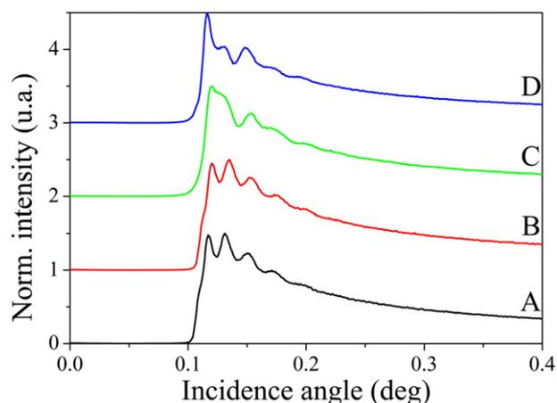
**Fig. 12.** Ag-K $\alpha$  GIXRF measurement of the IO/Ag/IO samples at 26,400 eV. Thinning of the top IO layer has greatly improved the sensitivity of the GIXRF technique. Differences in the GIXRF profile can be noted between the C (as deposited) and the D (annealed) sample.
