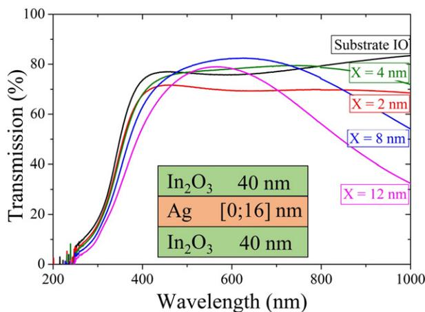
**Fig. 2.** Optical transmittance for IO/Ag/IO tri-layer samples with an Ag layer with varying thickness. For photovoltaic applications, the transparency in the visible is necessary and sample with an Ag thickness of 12 nm are not adapted.
