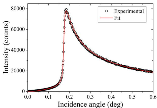
**Fig. 6.** GIXRF fit on JGIXA of a 50 nm Ni sample measured at 26,400 eV at ESRF. Fitting of reference sample allows the determination of geometrical factors such as the divergence of the beam and the size of the illuminated area.
