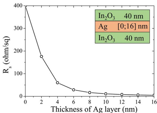
**Fig. 1.** Sheet resistance for IO/Ag/IO tri-layer samples with an Ag layer with varying thickness. 0 nm of Ag represents the sheet resistance of an 80 nm pure In<sub>2</sub>O<sub>3</sub> layer. For photovoltaic applications, acceptable sheet resistances have been obtained with Ag thickness superior to 4 nm.
