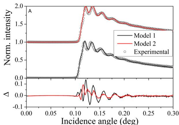
**Fig. 10.** Ag-K $\alpha$  GIXRF Gilda measurements and fits of sample A. The difference curve is represented at the bottom of the figure. Model 2 has been obtained by combining sets of data acquired at different excitation energies. It offers smaller differences between experimental and simulated data.
