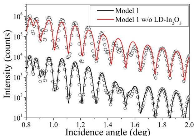
**Fig. 9.** XRR measurements (open circles) and fits (solid lines) of the as-deposited samples A at 8.05 keV with and without the introduction of the low-density  $\text{In}_2\text{O}_3$  top layer in the model. It can easily be seen that in order to reproduce the experimental data around  $1.5^\circ$ , the introduction of a low-density top layer is necessary.
