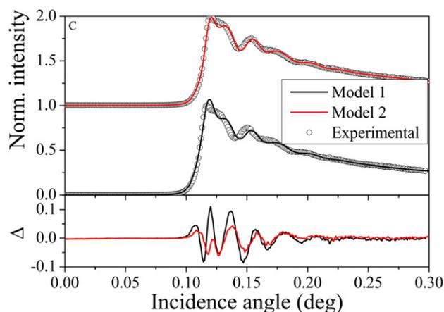
**Fig. 11.** Ag-K $\alpha$  GIXRF Gilda measurements and fits of sample C. The difference curve is represented at the bottom of the figure. Model 2 has been obtained by combining sets of data acquired at different excitation energies. It offers smaller differences between experimental and simulated data.
