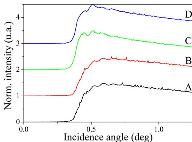
**Fig. 13.** Ag-L $\alpha$  GIXRF measurements of the IO/Ag/IO samples at 8050 eV. Thinning of the top IO layer has greatly improved the sensitivity of the GIXRF technique. Differences in the GIXRF profile can be noted between the C (as deposited) and the D (annealed) sample.
