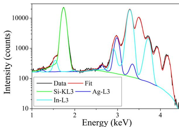
**Fig. 4.** Fluorescence intensity extraction from a measurement at 1.2° with a Cu-tube. Due to the correlation of Ag-L3 and In-L3 fluorescence peaks, the use of a third-party software like PyMCA [14] is necessary.
