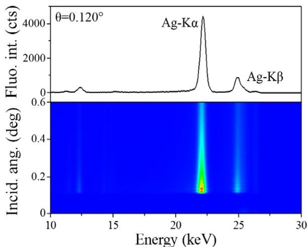
**Fig. 5.** Fluorescence intensity from a measurement at 26,400 eV with a synchrotron radiation at an angle of incidence  $\theta = 0.12^\circ$ . With this excitation energy, the fluorescence peaks of interest are not overlapping.
