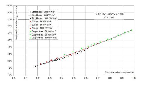
Fig. 4. Example of a SCS characteristic curve (Source: IEA SHC [5])
