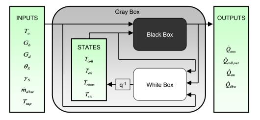
Fig. 3. Architecture of the "Gray Box" model proposed to model SCS behavior from SCSPT experimental results
