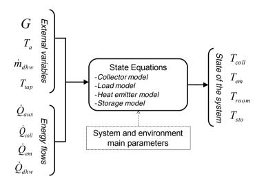
Fig. 2. Scheme of the "White Box" part
