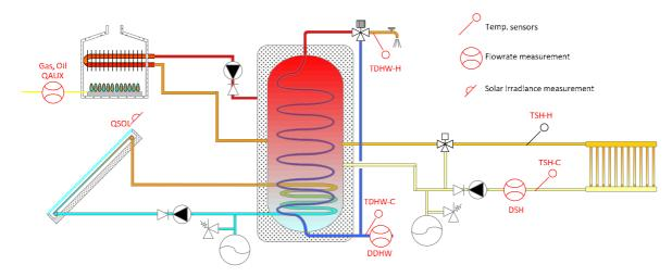
Fig. 1: Studied Solar Combisystem equipped with measuring instruments
