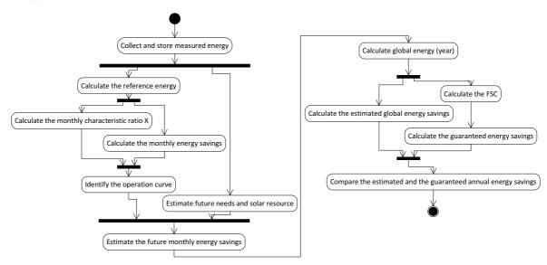
Fig. 3: Global diagram of the operations to be done monthly for the proposed monitoring procedure
