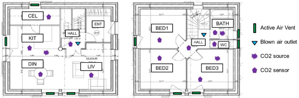
**Figure 5.** Introduction of the experimental house – Left: Plan of the first floor. Right: Plan of the second floor.
