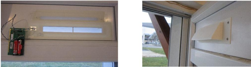
**Figure 2.** Pictures of one AAV prototype in the experimental house – Left: From inside, Right: From outside.
