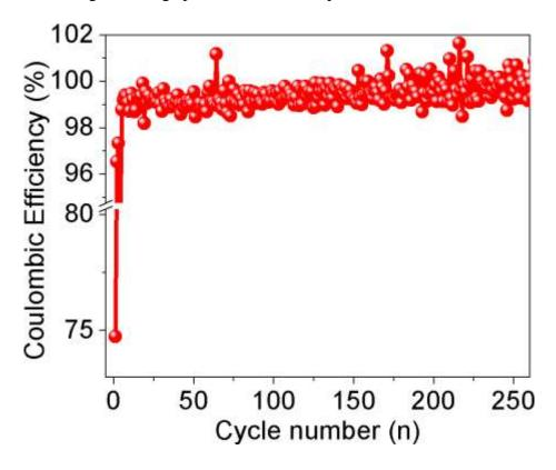
Figure S9. Coulombic efficiency behavior of Gt-SiNW at 2C.
