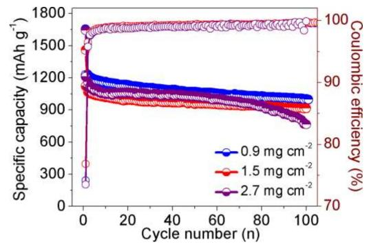
**Figure S11.** Specific capacity of Gt-SiNW anodes versus cycle number with different mass loadings from 0.9 to 2.7 mg cm<sup>-2</sup> at 0.2 C using 1 M LiPF<sub>6</sub> in 1:1 (v/v) EC: DEC with 2 wt% VC and 10 wt% FEC as electrolyte.
