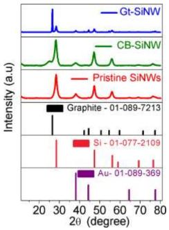
**Figure S4.** XRD pattern of pristine SiNWs, Gt-SiNW and CB-SiNW collected between 2theta 0 and 80. The number in the legend is referring to the ICSD card.
