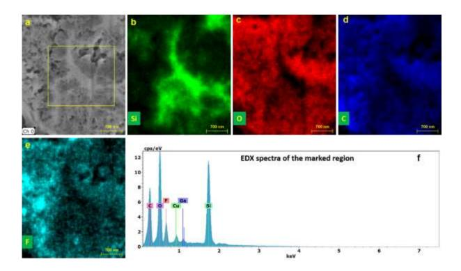
**Figure S15.** SEM-EDX chemical mapping of SiNW agglomerates in Gt-SiNW electrode after 200 cycles in the delithiated stage. b—e, individual mapping and distribution of elements Si, C, O and F. f, EDX spectrum averaged over of the yellow box in fig 9 a.
