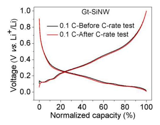
**Figure S10.** Charge-discharge profile (normalized only with galvanostatic capacity) of Gt-SiNW cycled at 0.1 C rate before and after C-rate test using 1 M LiPF<sub>6</sub> in 1:1 (v/v) EC: DEC with 2 wt% VC and 10 wt% FEC as electrolyte.
