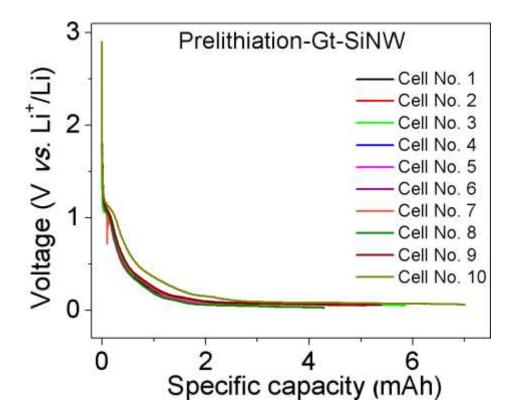
Discharge curve of Gt-SiNW anode cycled at 0.5 C rate using 1 M LiPF<sub>6</sub> in 1:1 (v/v) EC: DEC with 2 wt% VC and 10 wt% FEC as electrolyte during prelithiation.
