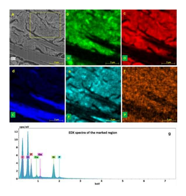
**Figure S16.** SEM-EDX elemental mapping of Gt-SiNW agglomerates/SEI region after 200 cycles in the delithiated stage. b—f, Elemental distribution of Si, C, O and F. g, EDX spectrum averaged over of the yellow box in Fig. 10 a.
