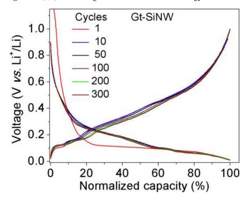
**Figure S6.** Charge-discharge profile (normalized only with galvanostatic capacity) of Gt-SiNW cycled at 0.2 C rate using 1 M LiPF<sub>6</sub> in 1:1 (v/v) EC: DEC with 2 wt% VC and 10 wt% FEC as electrolyte.
