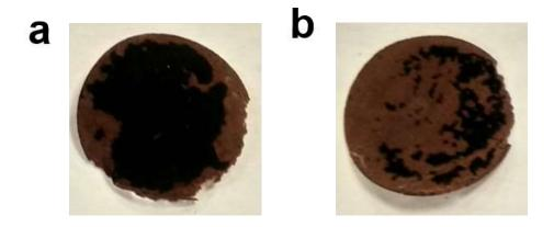
**Figure S14.** Photograph of CB-SiNW electrodes cycled at 0.2 C after (a) 100 and (b) 200 cycles, respectively.
