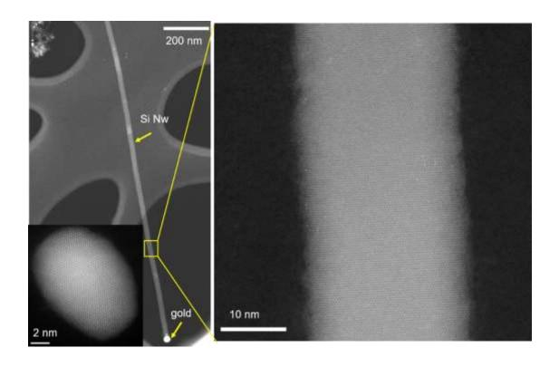
Figure S5. (a,b) STEM images of Gt-SiNW taken at an energy of 20 kV.
