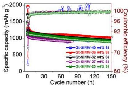
**Figure S2.** Electrochemical performance of several samples of Gt-SiNW with different Si wt% from 23 to 40 cycled at room temperature in half-cell configuration at 0.2 C rate using 1 M LiPF<sub>6</sub> in 1:1 (v/v) EC: DEC with 2 wt% VC and 10 wt% FEC as electrolyte.
