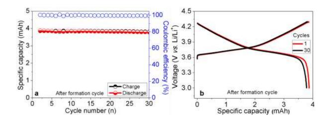
**Figure S20.** (a) Charge-discharge profile and (b) cyclability behavior of NMC-622 cathode investigated at a rate of 0.2 C rate between 3 to 4.3 V vs  $\text{Li}^+/\text{Li}$  using 1 M LiPF<sub>6</sub> in EC/propylene carbonate/dimethyl carbonate (v/v/v 1:1:1) as electrolyte.
