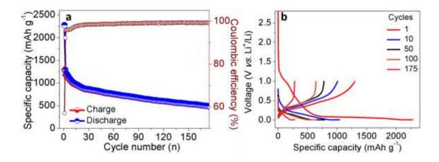
**Figure S12.** (a) Reversible charge/discharge capacity versus cycle number with corresponding Coulombic efficiency and (b) charge-discharge profile of CB-SiNW cycled at 0.2 C rate at room temperature in the 0.01-1.0 potential window and with 1 M LiPF<sub>6</sub> in 1:1 (v/v) EC: DEC with 2 wt% VC and 10 wt% FEC electrolyte.
