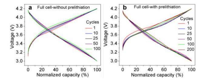
**Figure S19.** Charge-discharge profile (normalized only with galvanostatic capacity) of Gt-SiNW/NMC full cell (a) without prelithiation and (b) with prelithiation cycled at 0.5 C rate using 1 M LiPF<sub>6</sub> in 1:1 (v/v) EC: DEC with 2 wt% VC and 10 wt% FEC as electrolyte.
