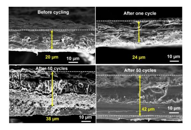
**Figure S13.** Cross sectional SEM view of Gt-SiNW electrodes (a) before cycling, and after 1 (b), 10 (c) and 50 (d) cycles at 0.2 C.
