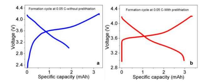
**Figure S18.** (a) Charge-discharge profile of the formation cycles of Gt-SiNW/NMC full cell (a) without and (b) with prelithiation cycled at 0.05 C rate using 1 M LiPF<sub>6</sub> in 1:1 (v/v) EC: DEC with 2 wt% VC and 10 wt% FEC as electrolyte.
