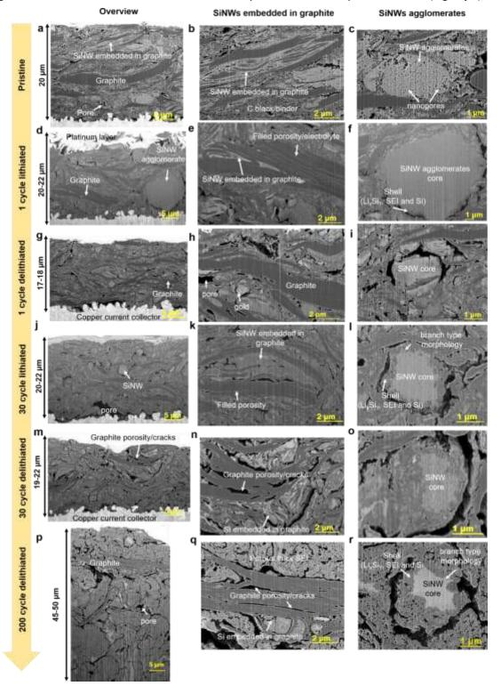
Figure 5. Morphological evolution upon cycling by cross-sectional FIB-SEM of Gt-SiNW electrodes: in pristine state (a), after 1 cycle lithiated (d) and delithiated (g), 30 cycles lithiated (j) and delithiated (m) and 200 cycles (p) in delithiated stage at 0.2 C rate. Corresponding high-resolution images of SiNWs embedded in graphite (b, e, h, k, n and q), and of SiNWs agglomerates (c, f, i, I, o and r) upon cycling.
