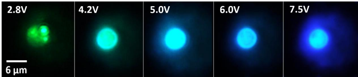
Figure 5. Optical photos of light emission on a 6\mu\text{m} diameter ‘green’ \mu LED at different bias values. The emitted wavelength is very dependent on applied voltage across the \mu LED. Green color turns to blue when increasing bias from 2.8V to 7.5V.
