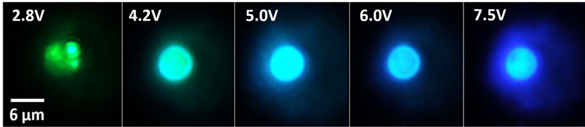
Figure 5. Optical photos of light emission on a 6\mu\text{m} diameter ‘green’ \mu LED at different bias values. The emitted wavelength is very dependent on applied voltage across the \mu LED. Green color turns to blue when increasing bias from 2.8V to 7.5V.
