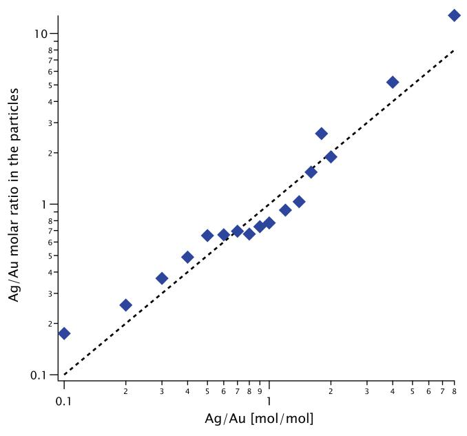
**Figure 7** The Ag/Au ratio in the particles, measured by ICP-MS, versus the same ratio in solution, K (diamonds). The dashed line marks the expected values if all the silver is deposited onto the gold cores.
