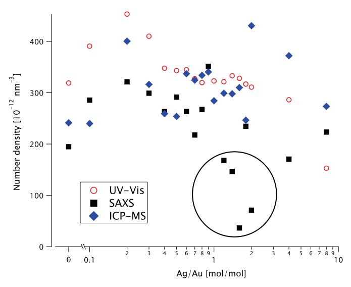
**Figure 8** Number particle density n as a function of the Ag/Au ratio K, extracted from fitting the SAXS data in Figure 3 (solid black squares), from the UV-Vis absorbance data (open red dots) and from ICP-MS (blue diamonds). Anomalously low SAXS values are circled.
