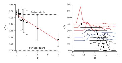
**Figure 2** Quadraticity parameter Q. Left: average value  $\langle Q \rangle$  as a function of K (mean and standard deviation, solid dots and error bars) with linear fit (solid line). The limiting values for a perfect circle and square are shown as dashed lines. Right: Histograms of Q for each K value (shifted vertically for clarity.) The mean and std. dev. from the left panel are shown under each curve. Colors (black, blue and red) distinguish three types of curves (see text.)
