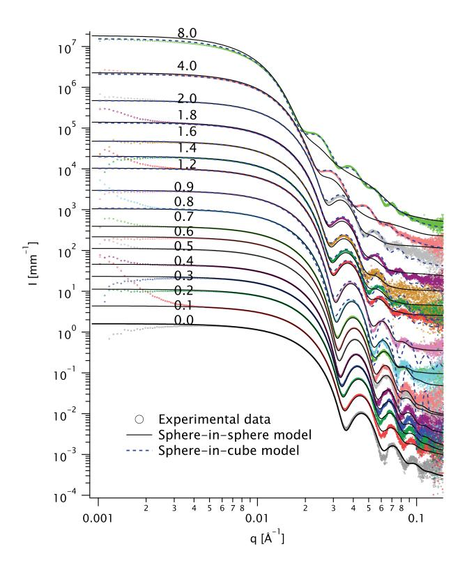
**Figure 3** Scattered intensity I as a function of the scattering vector q for all solutions (dots, various colors). The spectra were shifted vertically for clarity. The molar Ag/Au ratio K is indicated above each curve. Fits with the sphere-in-sphere model (solid lines) and with the sphere-in-cube model (dashed lines) are displayed for each curve.
