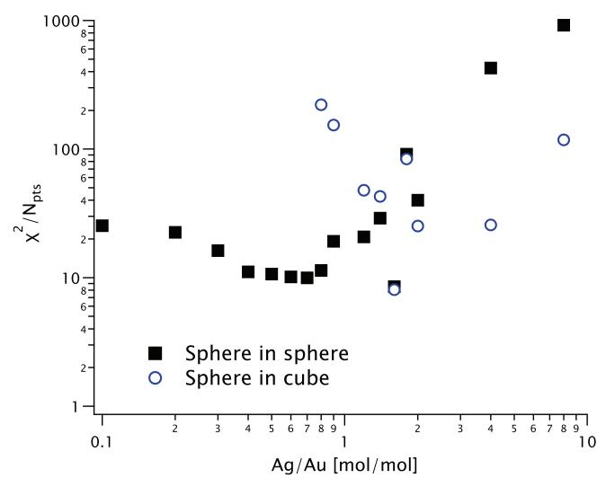
**Figure 4** Goodness-of-fit function for the SAXS models in Figure 3, shown as solid squares (for the sphere-in-sphere model) and as open circles (for the sphere-in-cube model) as a function of the Ag/Au ratio *K*.
