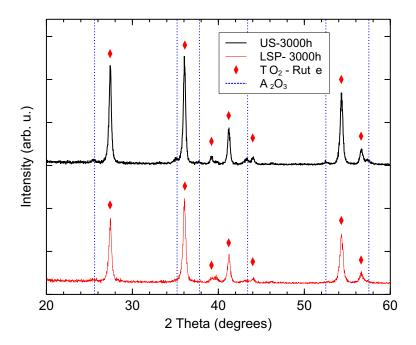
Figure 6: Grazing incidence XRD patterns of untreated (US) and laser treated samples (LSP) after oxidation at 700 °C during 3000 h. ICDS number of the compounds and phases identified in the pattern:  $\rm TiO_2$ -Rutile: 070-7347,  $\rm Al_2O_3$  (corundum): 070-5679.
