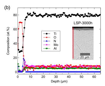
Figure S4: Variation in-depth of the atomic concentration of different elements (Ti, Al, Mo, O, N) measured by EDS in the cross-section of US and LSP samples after oxidation during 3000 h at 700  $^{\circ}$ C.
