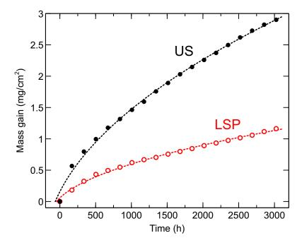
Figure 5: Mass gain curves of US and LSP samples during oxidation at 700  $^{\circ}$ C under synthetic dry air. Dotted lines correspond to the fitting of the experimental data to equation 1 with the parameters given in Table 1.
