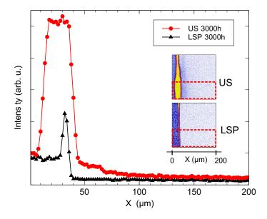
Figure 10: Oxygen depth profile in the US-3000h and LSP-3000h samples. The intensity of the oxygen signal in the DIGE maps of Figure 9 was summed at each depth X in the 40  $\mu$ m large rectangles (red delimited domains in the image) to increase the S/N ratio, and plotted as a function of depth (X).
