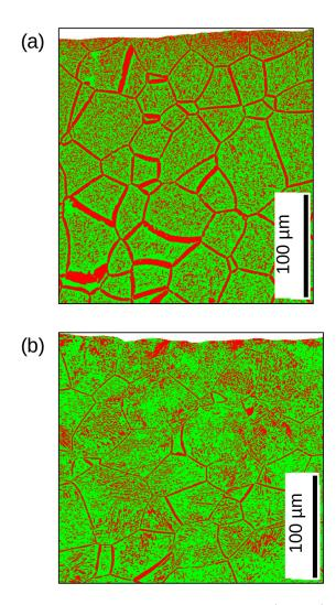
Figure 7: EBSD results showing the spatial distribution of  $\beta$ -Ti (in green) and  $\alpha$ -Ti (in red) phases in the cross section of (a) US-3000h and (b) LSP-3000h samples. The surface of the cross-sectioned sample is at the top of both images.
