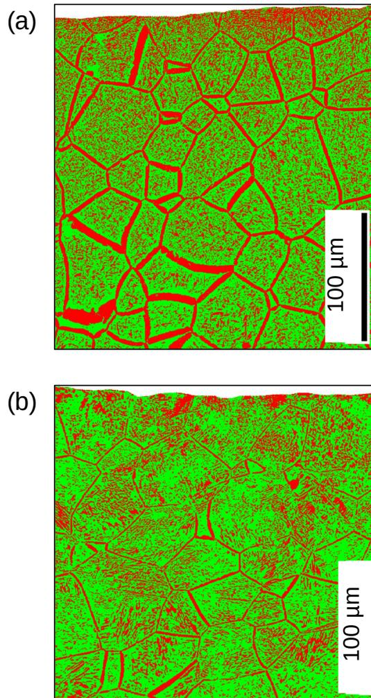
Figure 7: EBSD results showing the spatial distribution of  $\beta$ -Ti (in green) and  $\alpha$ -Ti (in red) phases in the cross section of (a) US-3000h and (b) LSP-3000h samples. The surface of the cross-sectioned sample is at the top of both images.
