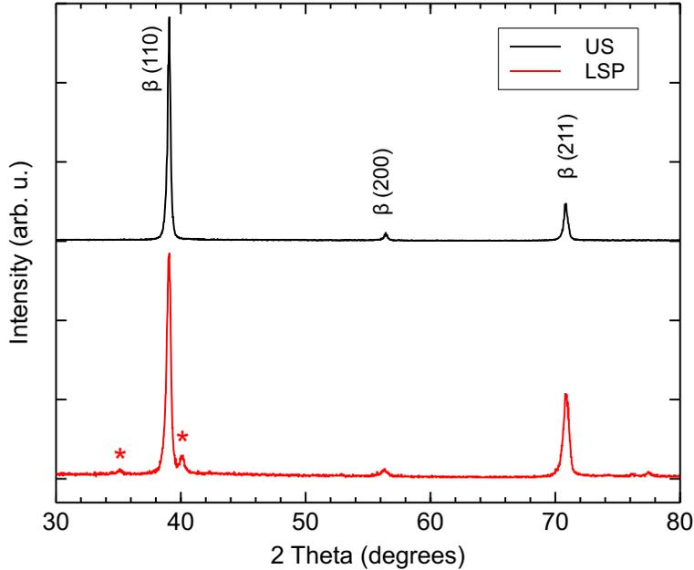
Figure 3: Grazing incidence X-ray diffraction patterns (incidence angle:  $2^\circ$ ) of untreated (US) and LSP treated samples. The peaks assigned to the  $\beta$ -Ti phase (ICSD: 0773482) are indicated. The intensity has been normalized to that of the  $\beta$ -Ti(100) reflection. The peaks tagged by stars (\*) have been tentatively assigned to the martensitic  $\alpha''$ -Ti phase.
