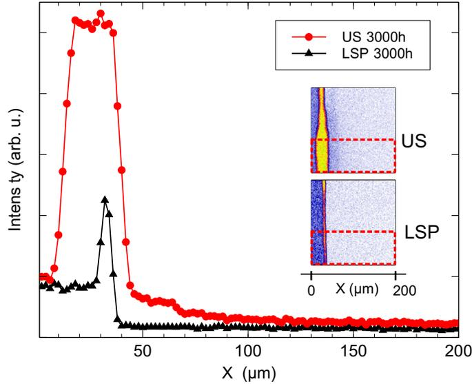
Figure 10: Oxygen depth profile in the US-3000h and LSP-3000h samples. The intensity of the oxygen signal in the DIGE maps of Figure 9 was summed at each depth  $X$  in the  $40 \mu\text{m}$  large rectangles (red delimited domains in the image) to increase the S/N ratio, and plotted as a function of depth ( $X$ ).
