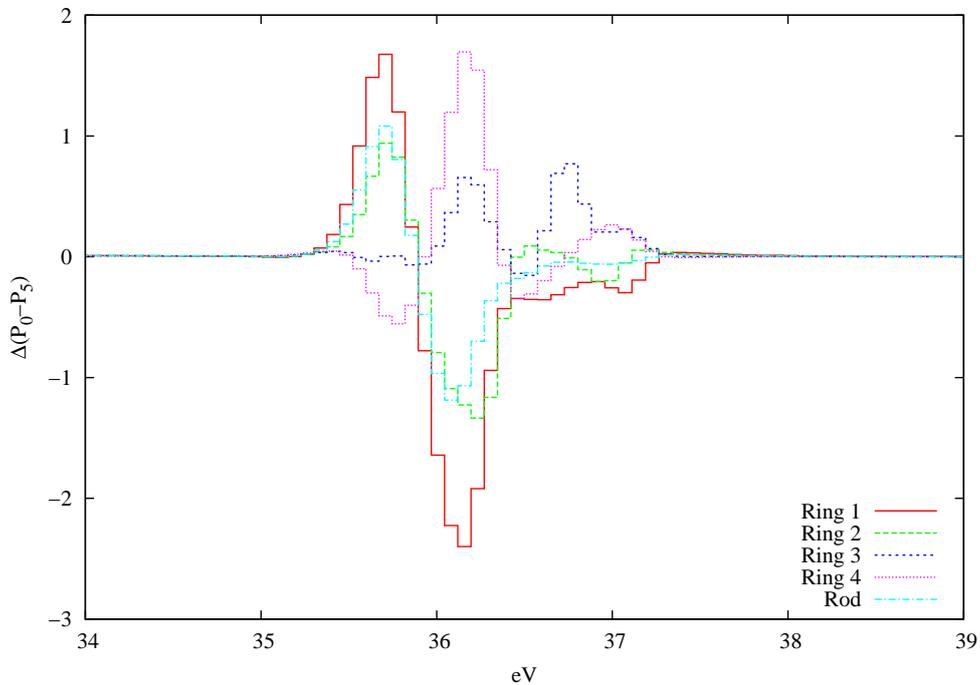
**Figure 11.** Differences  $\Delta(P_0 - P_5) = \left(\frac{AK-FG}{FG}\right)_{P_0} - \left(\frac{AK-FG}{FG}\right)_{P_5}$  on the  $^{238}\text{U}$  absorption discrepancy at 974 K between FG model and AK in the resonance at 36.68 eV
