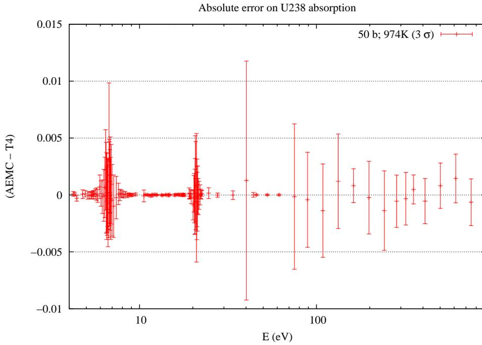
**Figure 4.** Differential discrepancies between AEMC and TRIPOLI-4 on the  $^{238}\text{U}$  absorption between 4 and 907 eV at 974 K and 50 barns
