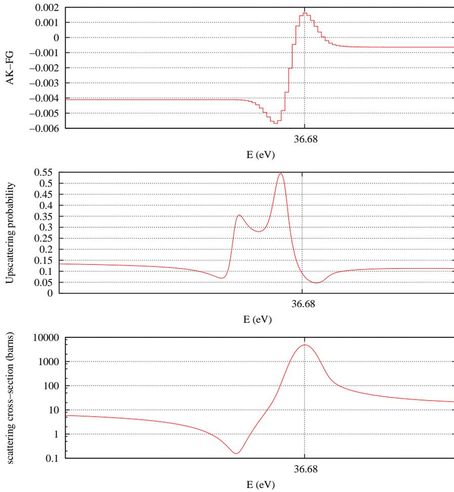
**Figure 7.** Relative cumulated error on absorption between asymptotic (AK) and free gas (FG) kernels at 50 barns and 974 K around the resonance at 36.68 eV. Below upscattering probability and scattering cross-section
