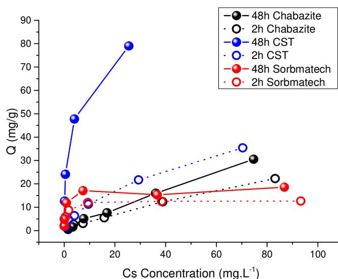
**Fig. 2.** Cesium sorption capacities (Q) of the three studied materials measured after 2 or 48 h in contact with seawater containing different concentrations of  $^{133}\text{Cs}$ . Sorbmatech, mesoporous silica functionalized with potassium-copper hexacyanoferrate nanoparticles; CST, crystalline silicotitanate.
