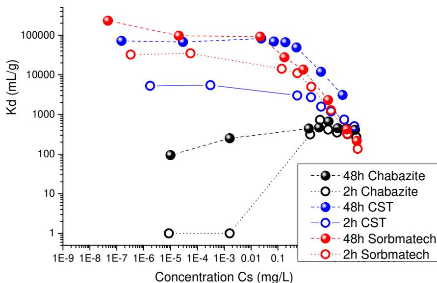
**Fig. 3.** Cesium distribution coefficients ( $K_d$ ) in the three studied sorbent materials measured after 2 or 48 h in contact with seawater containing different concentrations of either  $^{133}\text{Cs}$  (2-100  $\text{mg}\cdot\text{L}^{-1}$ ) or  $^{137}\text{Cs}$  (trace levels). Sorbmatech, mesoporous silica functionalized with potassium-copper hexacyanoferrate nanoparticles; CST, crystalline silicotitanate.
