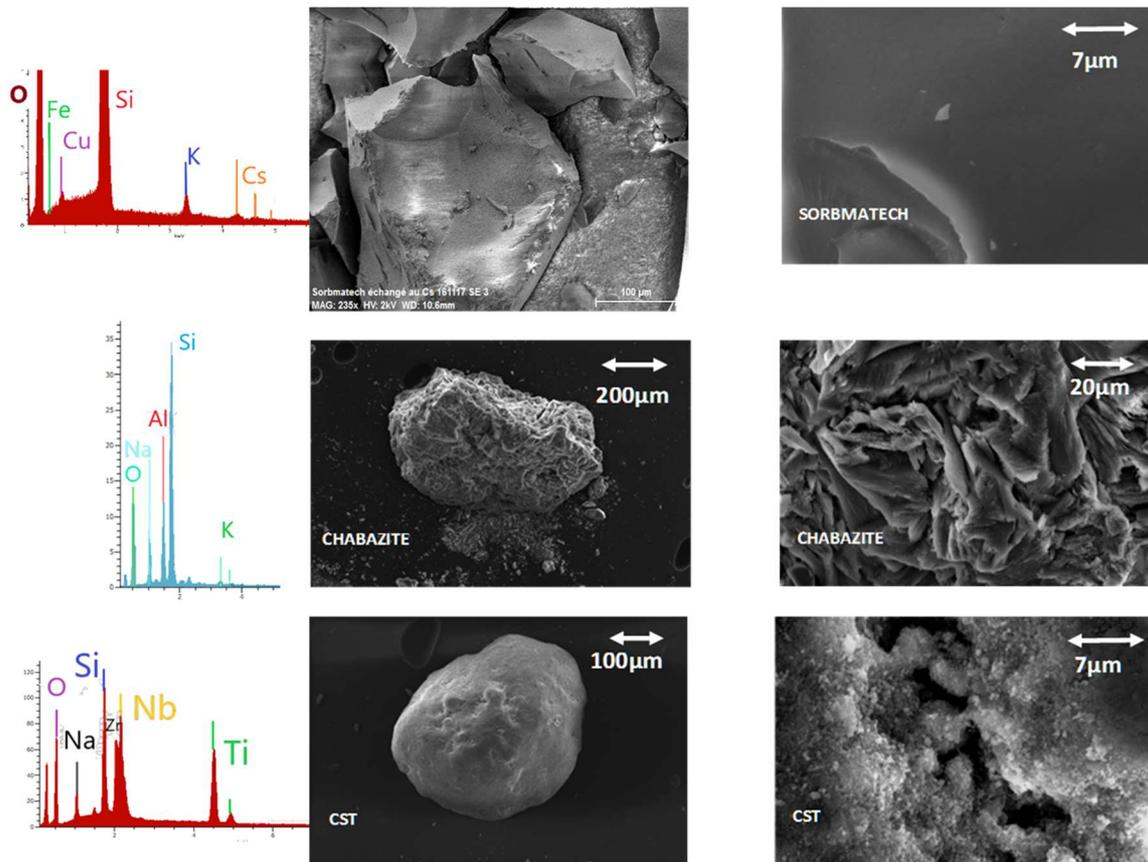
**Fig. 1.** Scanning electron micrographs and EDX analysis of the three sorbent materials investigated in this study: Sorbmatech (mesoporous silica functionalized with potassium-copper hexacyanoferrate nanoparticles), chabazite and a Nb-substituted Na crystalline silicotitanate (CST).
