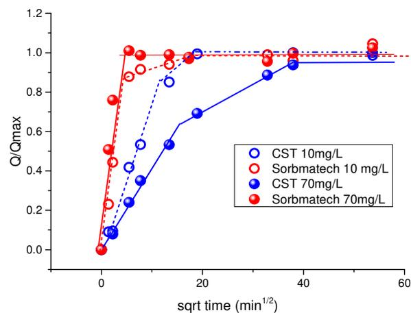
**Fig. 6.** Comparison of the (square-root) time-variation of the normalized cesium sorption capacities of Sorbmatech (mesoporous silica functionalized with potassium-copper hexacyanoferrate nanoparticles) and CST (a crystalline silicotitanate) in seawater containing 10 or 70  $\text{mg}\cdot\text{L}^{-1}$  Cs.
