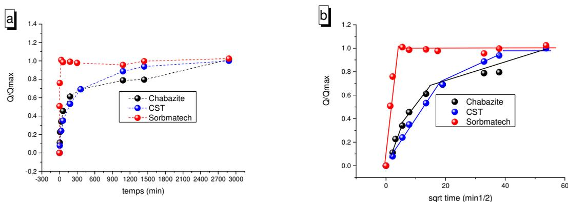
**Fig. 5.** Normalized cesium sorption capacities of the three studied materials as a function of (a) linear and (b) square root time as measured from batch experiments in seawater containing 70  $\text{mg}\cdot\text{L}^{-1}$  Cs. Sorbmatech, mesoporous silica functionalized with potassium-copper hexacyanoferrate nanoparticles; CST, crystalline silicotitanate.
