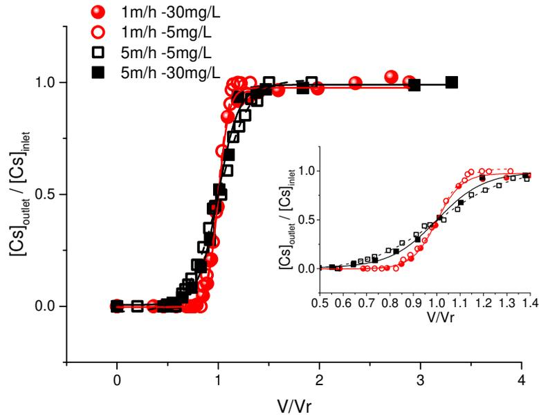
**Fig. 8.** Comparison of the breakthrough curves ( $[Cs]_{\text{outlet}}/[Cs]_{\text{inlet}}$  vs. ejected/retention volume) measured for Sorbmatech (mesoporous silica functionalized with potassium-copper hexacyanoferrate nanoparticles) at Darcy velocities of 1 and 5  $\text{m}\cdot\text{h}^{-1}$  and inlet  $C_s$  concentrations of 5 and 30  $\text{mg}\cdot\text{L}^{-1}$ . The retention volume,  $V_R$ , was calculated by fitting the experimental data using Eq. 7.
