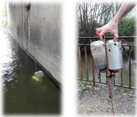
Figure S2 Sediment traps used in the study composed of PET plastic bottles drilled at their base to collect SPM by sedimentation. The plastic bottles were used for TE analysis in SPM.
