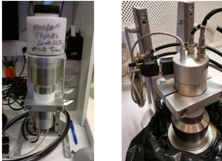
Fig. 17. Photographs of the beta spectrometer for measurements on sand samples in a standardized container (bottom left) and in direct contact with the sand (bottom right).
