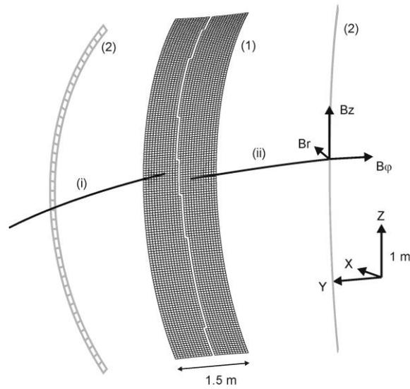
Fig. 1 : Component mesh Ecomp (1, in black) and shadowing mesh Eshad (2, in gray). Eshad is the central ridge of Ecomp, rotated from  $\pm 20^\circ$  degrees. Two field lines are represented, (i) escapes the shadowing mesh, and the node of Ecomp from which it originates is designed as wetted, whereas (ii) connects to neighbour limiter, so that the the node of Ecomp from which it originates is designed as shadowed.
