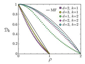
FIG. 7: Coefficient of self-diffusion vs density for the SEP in two and three dimensions, and for the GEP with k=2 in dimensions d=1,2,3. Dots represent simulation results. Solid lines are the mean-field predictions:  $\mathfrak{D}_1^{\mathrm{MF}}=1-\rho$  for the SEP, while for the GEP with k=2 the mean-field prediction  $\mathfrak{D}_2^{\mathrm{MF}}=\Lambda_2(\rho)$  acquires the explicit form (26).
