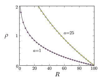
FIG. 4: Stationary density profiles versus R for the GEP with k=2 in the annulus with external radius L=100. Dots are simulation results which were obtained by averaging over  $5 \times 10^6 \le t \le 10^7$ . Solid lines are theoretical predictions given by (37) with  $\alpha=1/4$  in the case of a=25 and by (38) when a=1.
