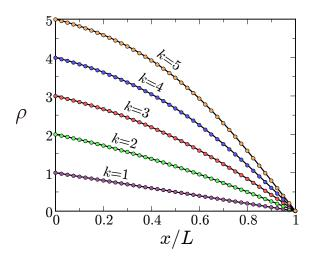
FIG. 3: Stationary density profiles versus x/L for the GEP with k=1,2,3,4,5 on a segment with  $L=10^3$ . The solid lines are theoretical predictions in the case of extremal boundary densities,  $\rho_0=k$  and  $\rho_1=0$ . For the SEP (k=1), the density profile is linear; for k=2, the density profile is given by (33), and generally it is extracted from Eq. (35). Simulation results (shown by  $\bullet$ ) were obtained by averaging over the time window  $5\times 10^6 \le t \le 10^7$ .
