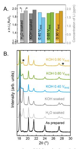
**Figure 2:** (A) The concentration of Li ions in the solution after exposure of  $Li_2RuO_3$  pellet (50 mg) to water, 0.1 M KOH and after holding at three potentials (0.40, 0.65 and 0.90) in 0.1 M KOH for 24 h, measured by inductively coupled plasma mass spectrometry, and corresponding lithium stoichiometry present in  $Li_xRuO_3$ . (B) Parts of the X-ray powder diffraction data of pellets after exposure described in (A) ( $CuK_\alpha$  radiation, full patterns are shown in Figure S5).
