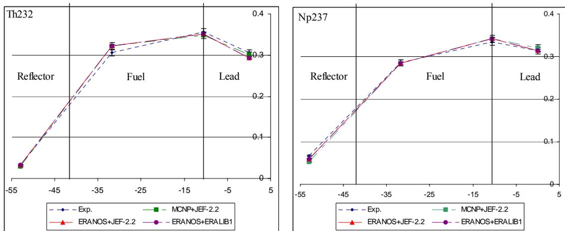
Figure 2. Np<sup>237</sup> and Th<sup>232</sup> fission rates along the west/east axis (The sum of the ordinates is normalised to 1.0 in each case.)
